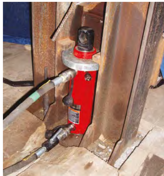
HD cylinders can be used in pushing and pulling applications. In this photo, we see a HD cylinder set up for a pull application using a Plunger Clevis cylinder accessory
